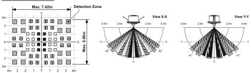
The X-Y cross-sectional diagram shows the detection area. The differences in the detection zone patterns indicate the projections of the 16 lenses with a single focal point. Movement of an object with higher than background temperature, between the detection zones, will be detected.
